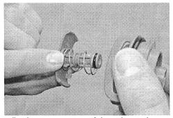
Pull valve actuator out of the valve and remove spiral spring.
