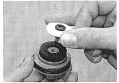
Insert rubber disk - screw valve actuator together with plastic screw (see photo). Insert valve in the cassette again
