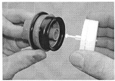
Press in valve actuator - press float against sealing lip and turn anticlockwise.
